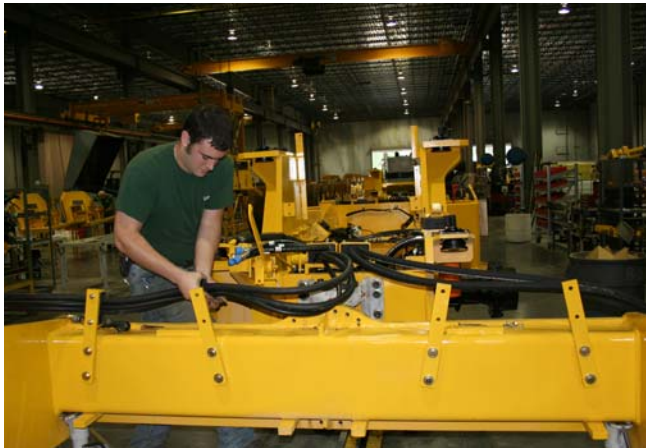
Sakai America technician routes hydraulic hoses for the company's 1000th roller, and SV-505D.
