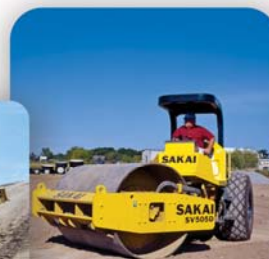
Vibratory Soil Compactors
