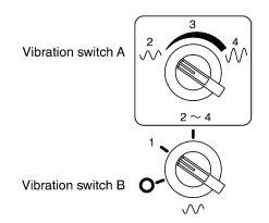
Tilting the lever again resets the amplitude to the selected one of 2 to 4.
