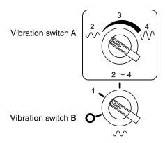
When the F-N-R lever is placed in the neutral position N during rolling compaction work at vibration 2 to 4, return is made to the amplitude of vibration 1. Tilting the lever again resets the amplitude to the selected one of 2 to 4.
