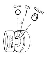
The engine is preheated automatically when it is cold. Hold the key in this position until the lamp on the monitor display goes out.
