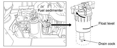
**NOTE**: After purchasing a new machine, drain water 50 hours after the initial operation.
