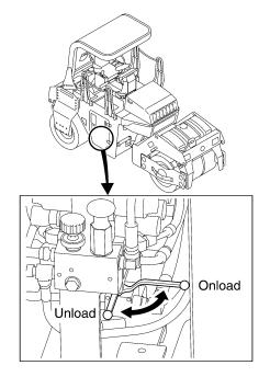
**NOTE**: For normal travel, be sure to hold the valve in the ONLOAD position.
