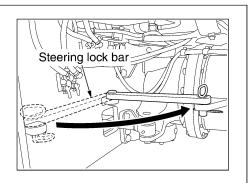
1) Put wire ropes securely on the hook and lifting points as shown.
