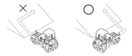
■ On a steep slope, run the machine at low speed
