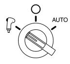
**NOTE:** Vibratory compaction is not possible when the engine speed selector switch is in the IDLE position.
