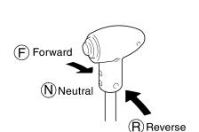
**NOTE:** When the F-N-R lever is not in the neutral position  $\textcircled{\mathbb{N}}$ , or the parking brake has been released, the interlocking system goes into operation and the engine will not turn on. Be sure to confirm that the F-N-R lever is in the neutral position  $\textcircled{\mathbb{N}}$ , and that the parking brake is engaged before starting the engine.
