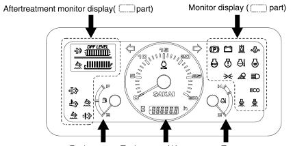
Fuel gauge Tachometer / Hour meter Temperature gauge
