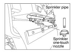
3) Clean the filters. Use a needle or the like to clean nozzle hole. Refit the filters to the nozzles.
