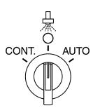
The indicator lamp  $\frac{1}{2}$  on the monitor display will turn on only while water is being sprinkled.
