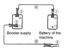
Connect to the engine block earth of the machine
