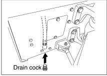
2) Refit the drain plug and fill the crankcase with the engine oil from the fill hole on the cylinder head cover.
