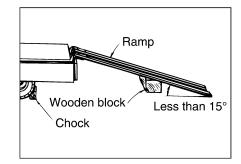
Decide the correct direction of run and conduct loading or unloading at low speed.
