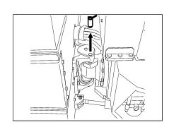
**NOTE**: Mount the removed lock pin in the innermost section of the step at the left of the machine.
