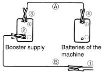
Disconnect from the engine block earth of the machine
