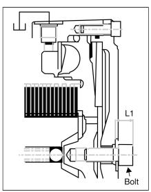
3) Inspection of brake stroke
