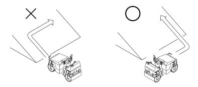
On a steep slope, run the machine at low speed
