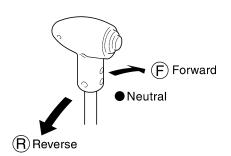
**NOTE:** The travel speed can be controlled by the throttle lever and F-N-R lever.
