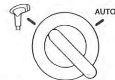
Vibration selector switch (C)
