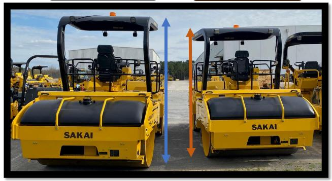
The Low Profile ROPS reduces the overall height of the freight during transportation ... good for communities with older bridges and infrastructure
