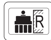
Right side wall compaction mode mark
