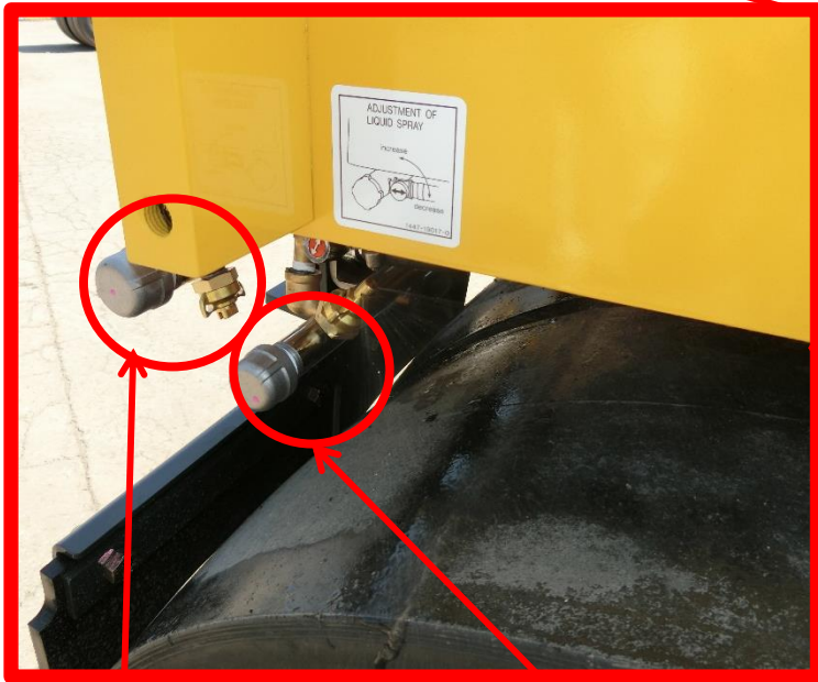
Water spray tank
